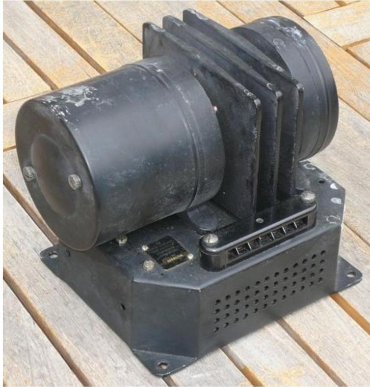
**Carbon pile mechanical regulator**
