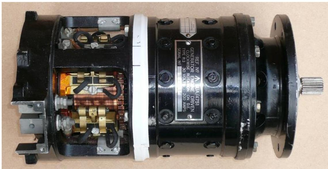
**Typical aircraft DC generator gas turbine driven**
