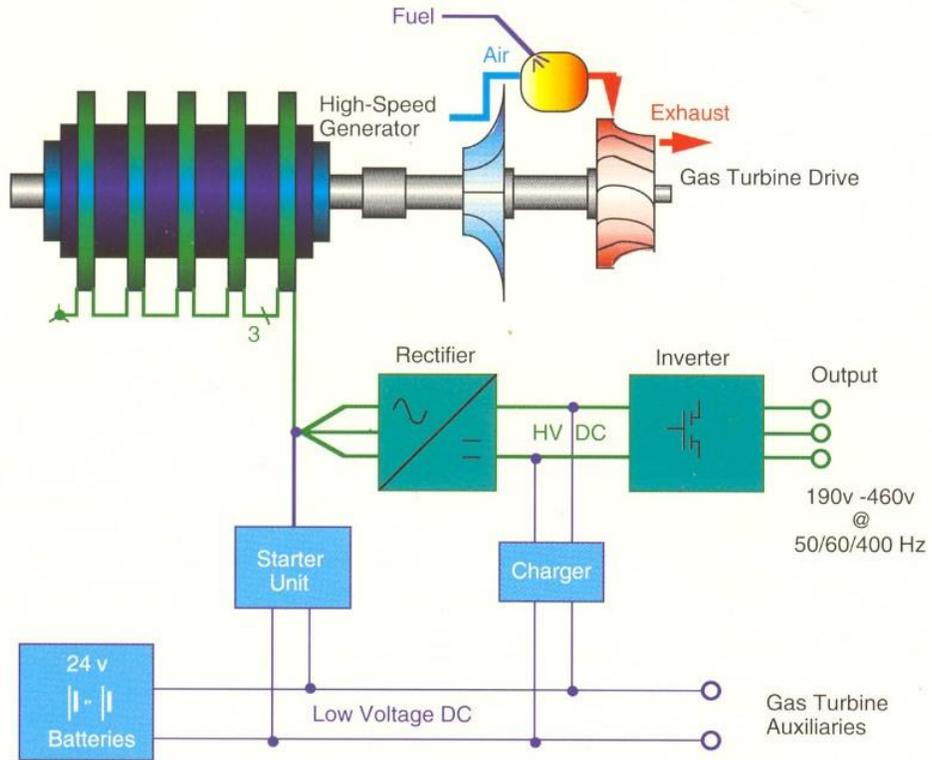
**System diagram of a direct drive gen-set**
