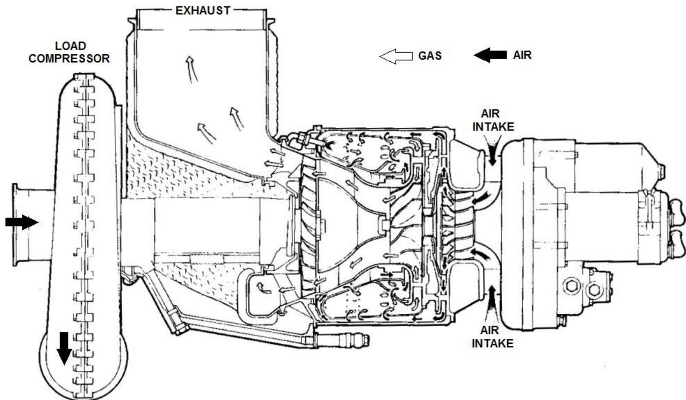
**A twin-shaft gas turbine compressor unit (Rover AAPP MK10501)**
