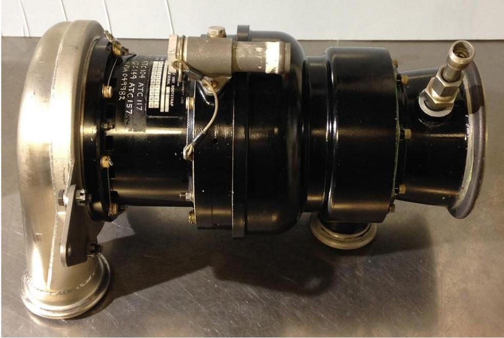
**A Cold Air Unit (CAU) Air Cycle Machine**
