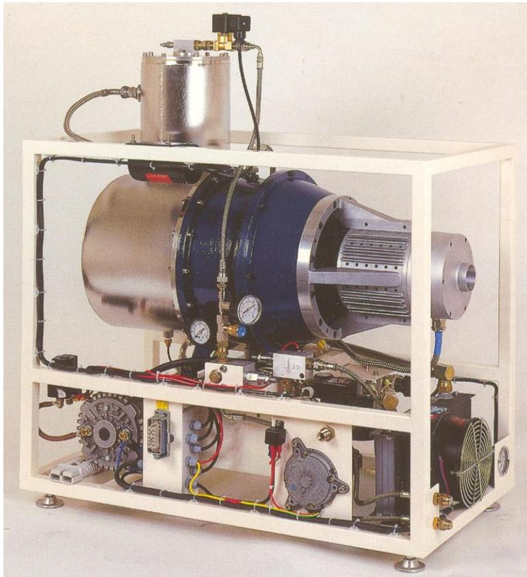
**Experimental direct-drive gas turbine generator**
