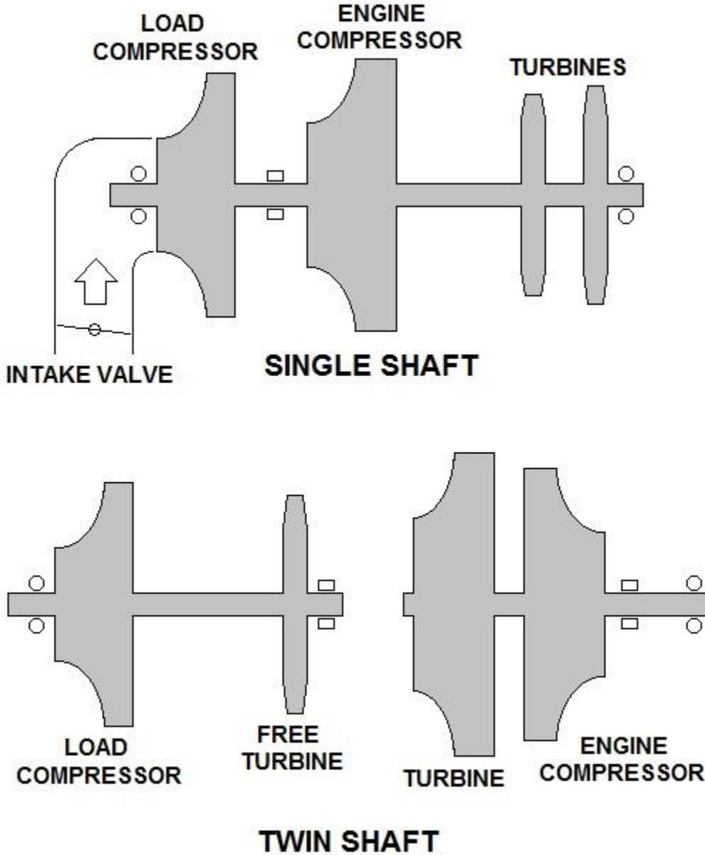
**Load compressors; single shaft and twin shaft gas turbine driven**
