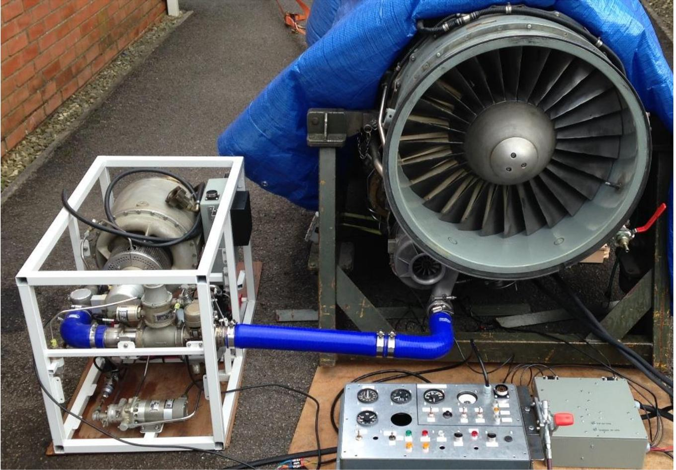
**Installed air motor (starter) mounted on an engine and fed from an APU**
