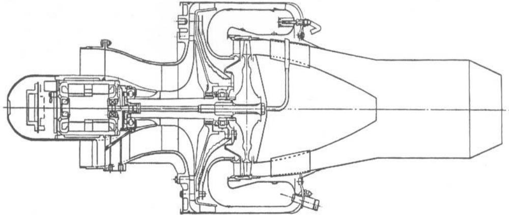
**High speed alternator fitted to turbojet engine (NPT301)**
