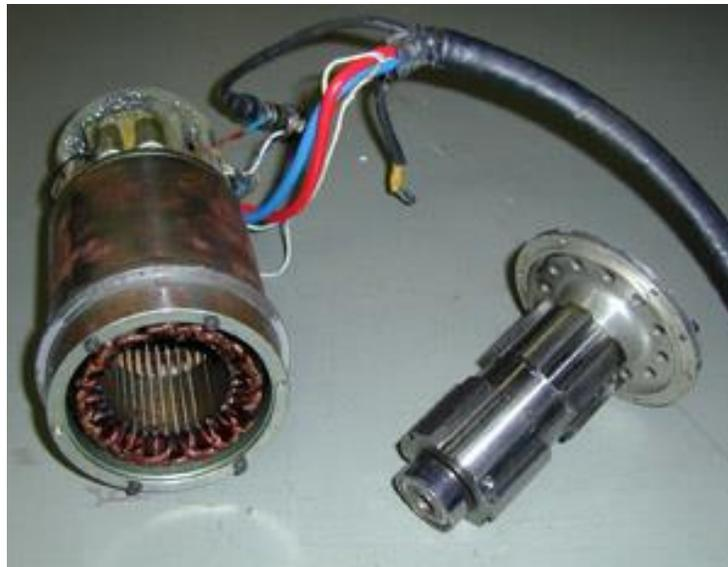
**High speed alternator components (stator and rotor)**
