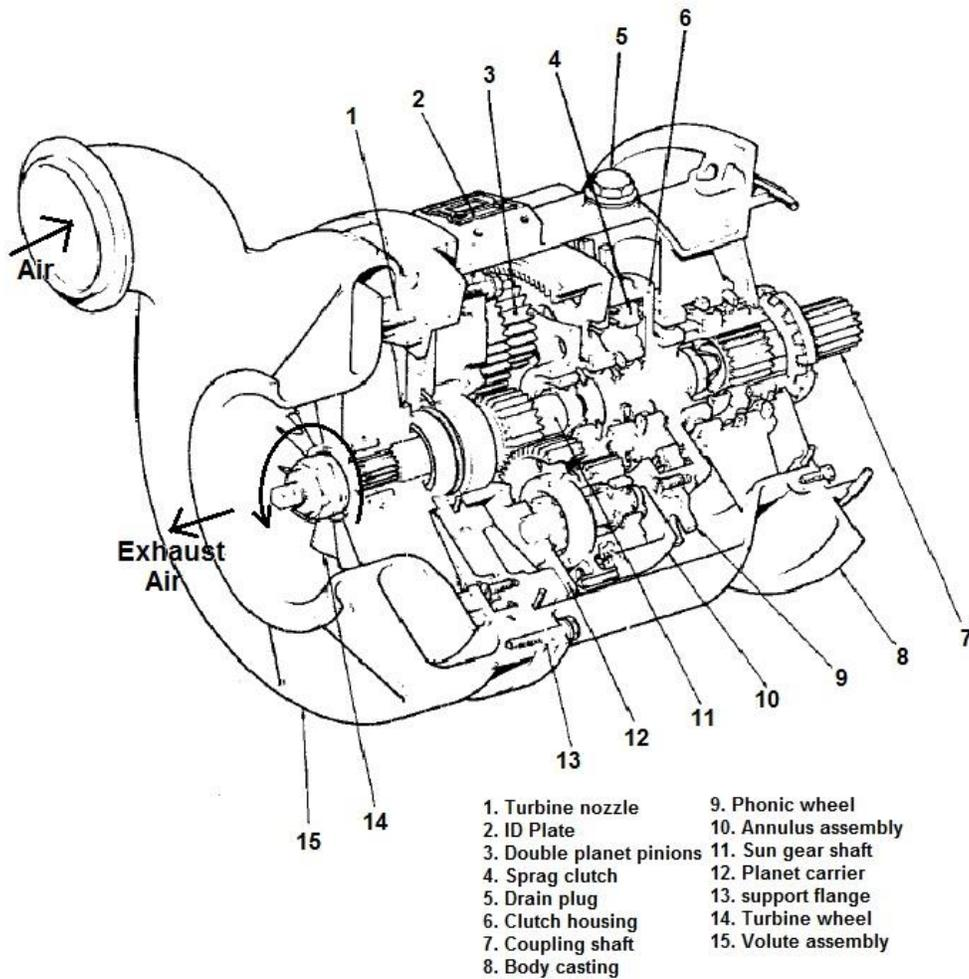
**Air turbine motor unit (Microturbo air-starter)**
