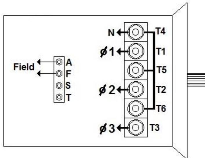
**Plessey 30KV<sub>a</sub> 400Hz brushless alternator connections**
