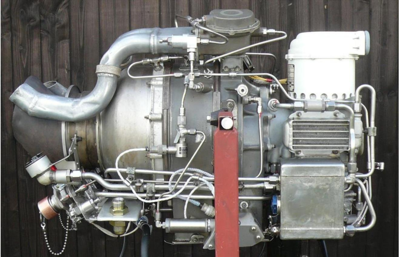
**Single-shaft gas turbine engine with separate driven compressor (Williams WR27 APU)**
