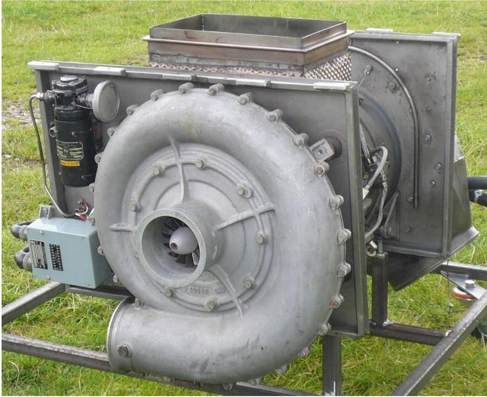
**Engine driven centrifugal compressor unit (Twin Shaft)**
