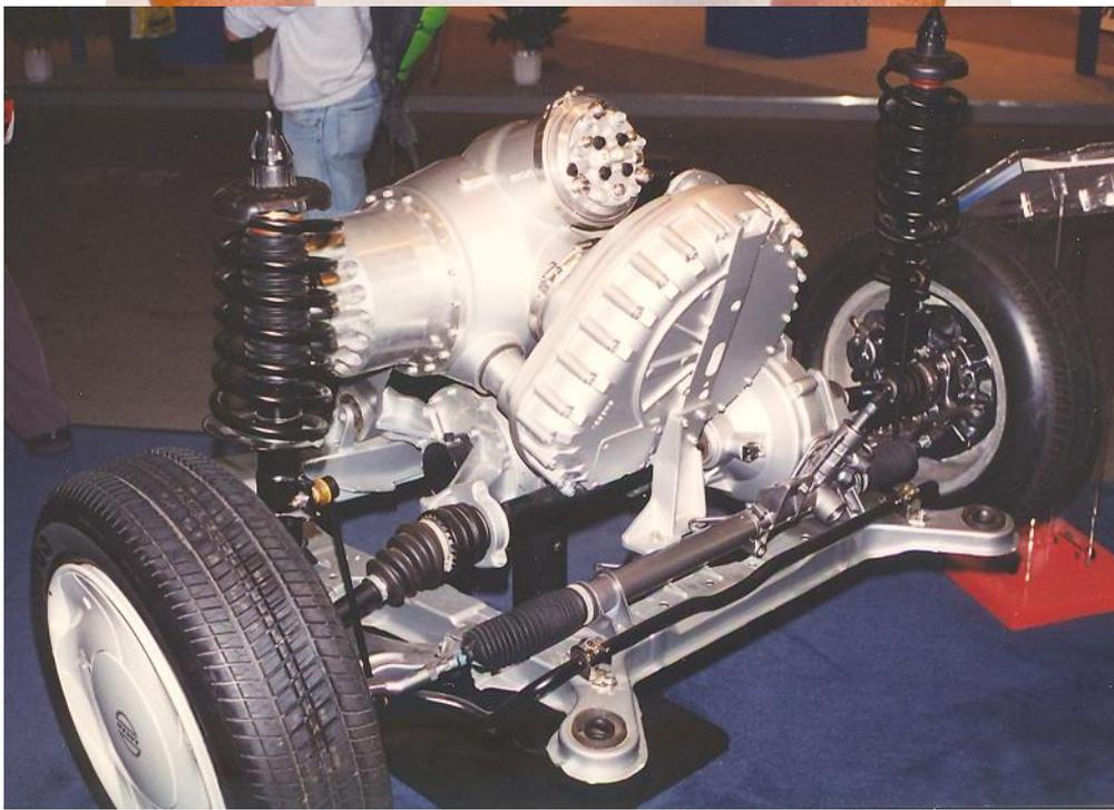
**Automotive gas turbine with direct-drive alternator and recuperator**
