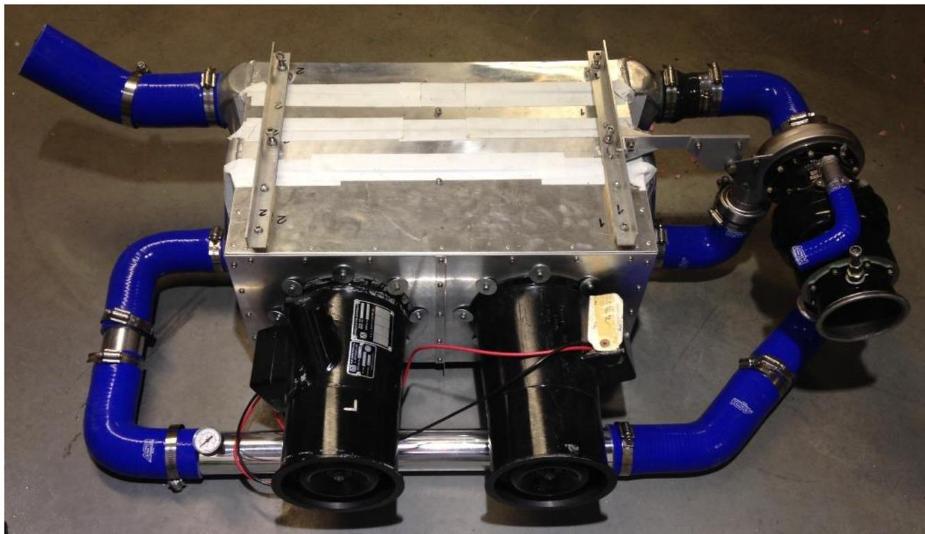
**Air cycle cooling pack built with automotive intercoolers**
