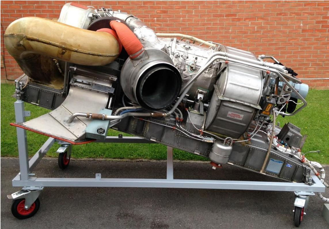
**Pratt and Whitney PT6 (ST6L73) derived twin shaft unit driving a load compressor**
