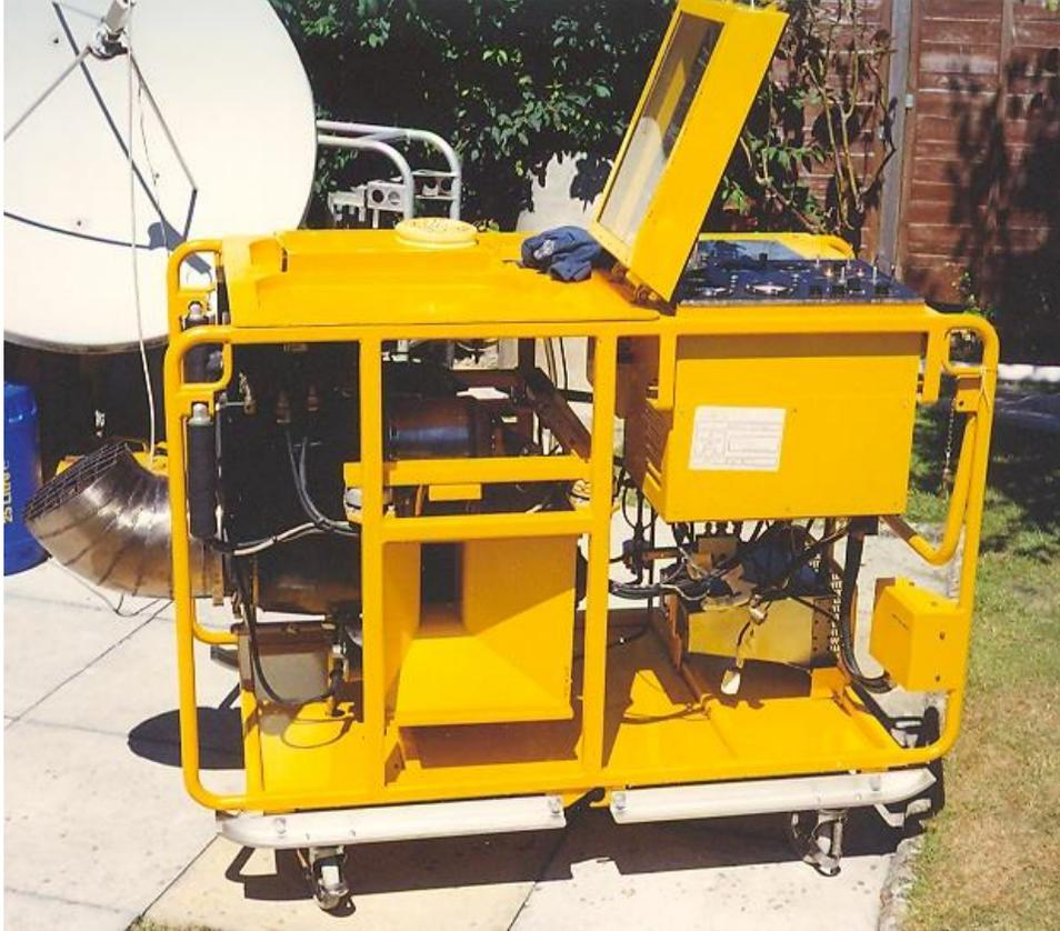
**Air portable 500A 28V DC generator set (Rover 1S60)**
