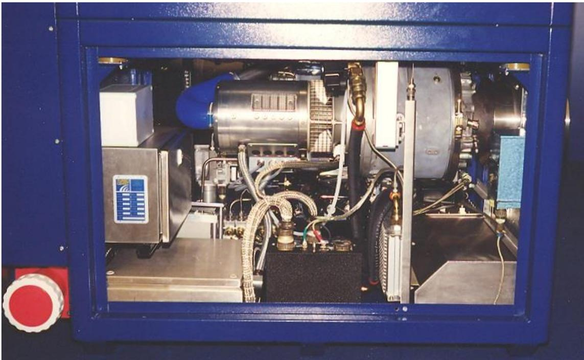
**High speed direct drive generator set with 50Hz output (Turbogenset)**
