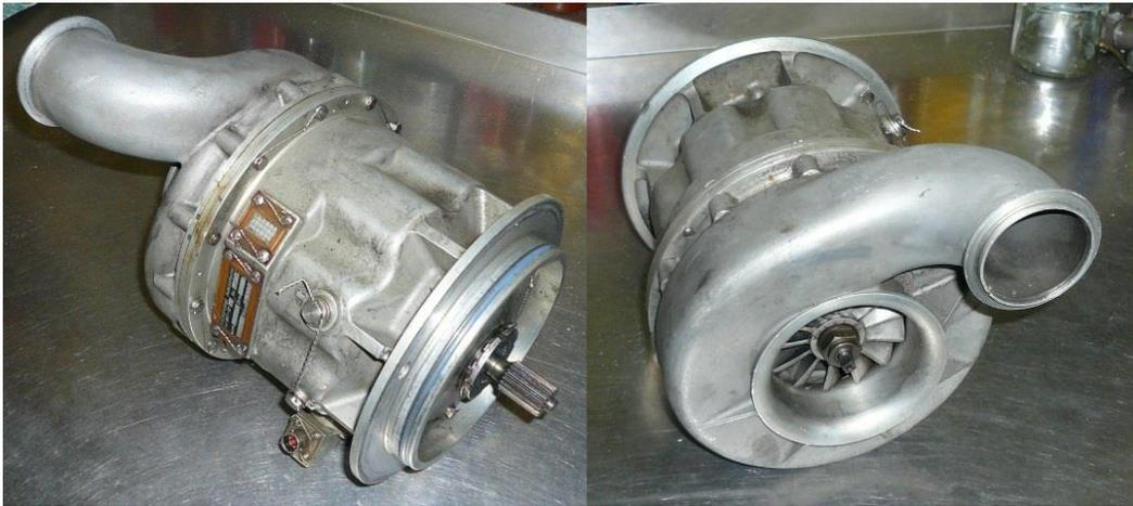
**LP air driven starter turbine unit (Microturbo)**
