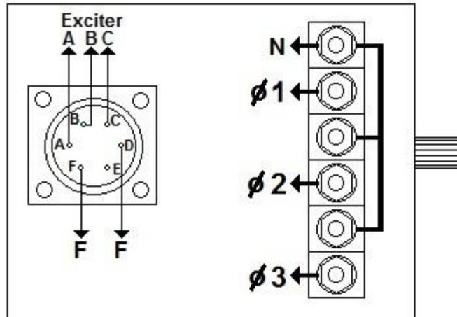
**Bendix 25KV<sub>a</sub> 400Hz brushless alternator connections**
