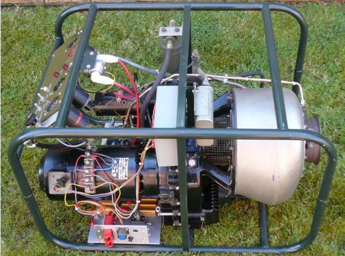
**Portable 25 KVa gas turbine driven generator set**
