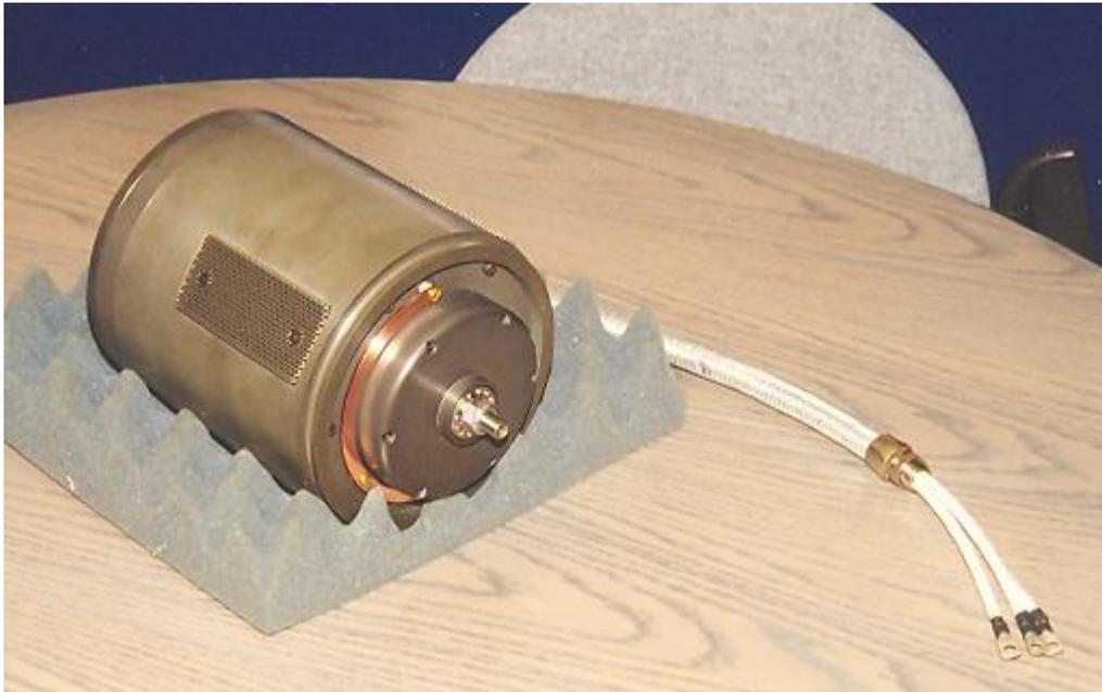
**High speed alternator (Turbogenerator)**
