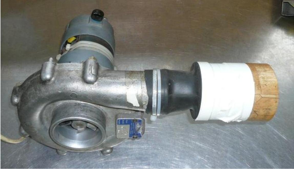
**Motor driven blower unit used for starting**
